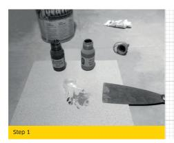
Use a Neolith fragment to imitate the surface finish and fill the defect with the mixed resin.
